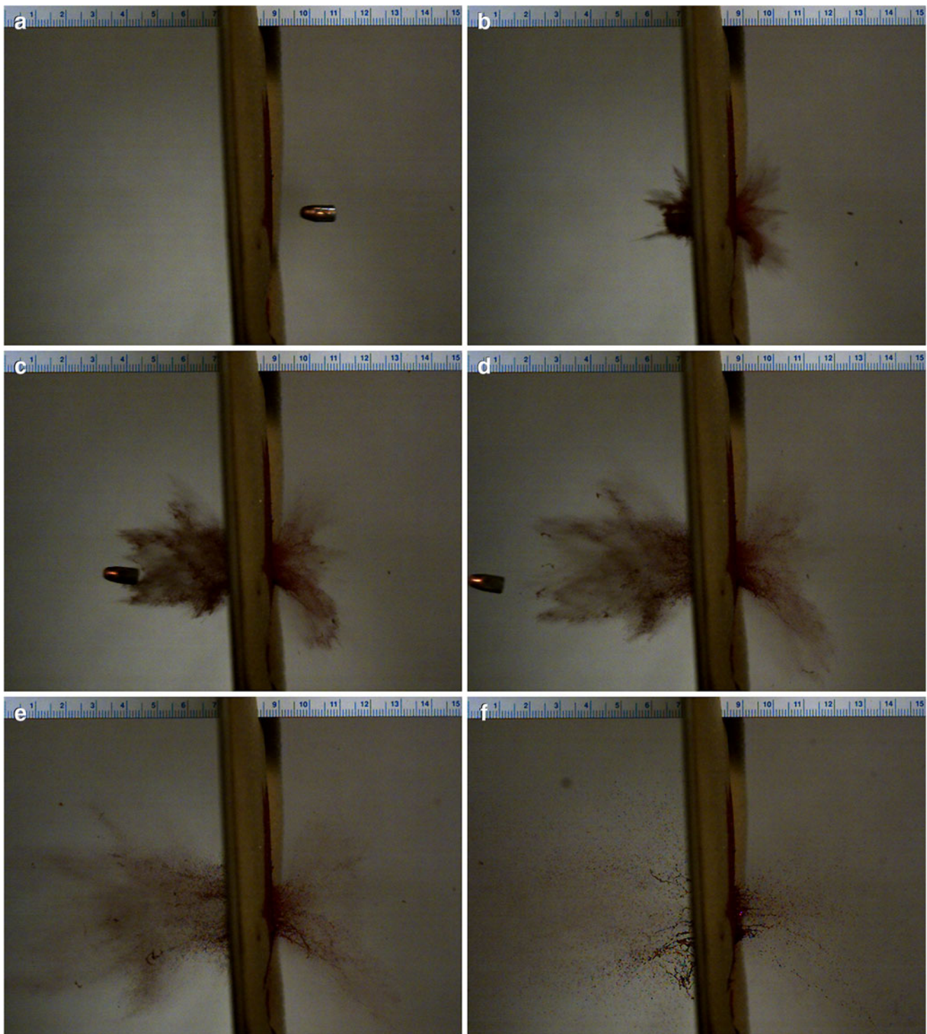
Fig. 5 Sequence of images of the impact of a .22 caliber bullet that has passed through an intermediate target (not shown) before striking a bloodied sponge. a t = -0.1 ms. b t = 0 . Impact of the bullet with the
